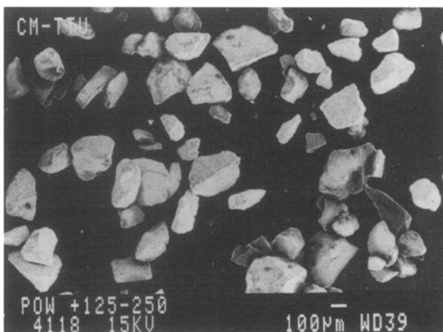
Fig. 2 Micrograph of WC-15% Co powder from +125–250 \mu\text{m}
